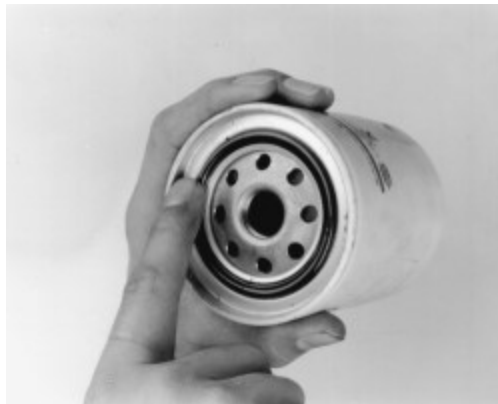
Fig. Coat the gasket on the new filter with fresh engine oil. Partially filling the new filter with oil will reduce the time the engine must run dry on start up
