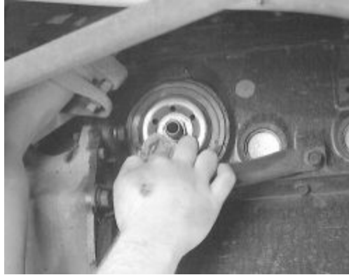
Fig. Be sure to clean the mounting boss' gasket surface before installing the new filter
