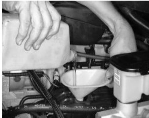
Fig. Even with "easy pour" bottles, it is still wise to use a funnel to keep oil from spilling
