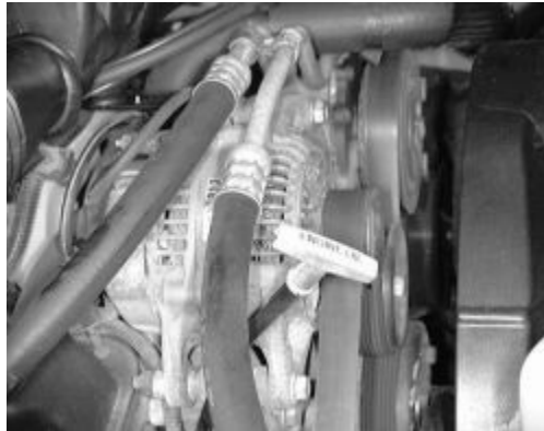
Fig. Dipstick handles are marked for application
