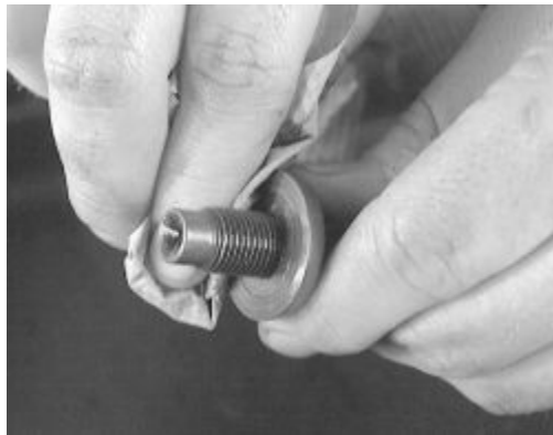
Fig. Be sure to clean and inspect the drain plug threads. Do NOT reuse self-tapping bolts
