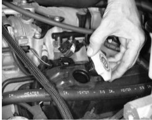
Fig. On some models, remove the oil filler cap from the rocker arm cover to add oil
