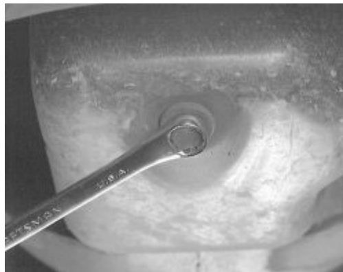
Fig. Loosen the oil drain plug with a wrench, and then carefully remove it with your fingers
