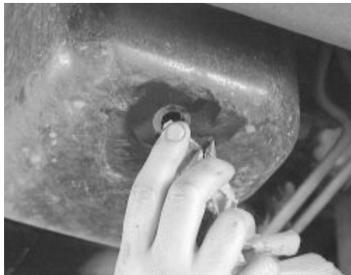
Fig. Be sure to clean and inspect the drain plug threads. Do NOT reuse self-tapping bolts
